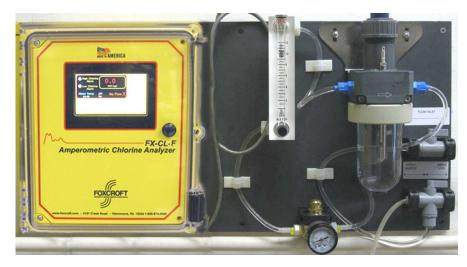
The Foxcroft FX-CLF amperometric reagentless free chlorine residual analyzer reliably measures continuously without moving parts in a variety of applications with clean filtered water of drinking or swimming pool quality.
