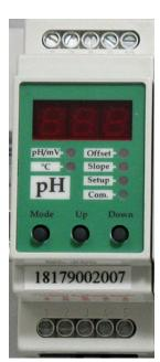
**"Buffer"** is the calibration mode for the offset or high pH solution. Use the Up or Down keys to adjust after the software is unlocked.
