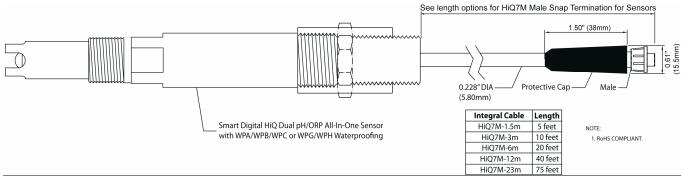
Detail drawing for standard female snap to tinned leads cable extensions Dual pH/ORP sensors:
