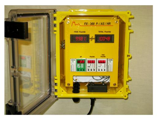
While our fluoride sensor is published to measure up to 19,000 ppm, or 1 Molar ion activity, the sensor is actually capable of measuring up to saturation. While the sensor can measure up to 100,000 ppm, there are special considerations and extra work required to calibrate above 19,000 ppm due to a variety of physical chemical issues such as activity coefficients as well as some reduced slope at elevated concentration that is inherent to this or any ISE sensor.
