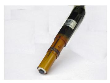
Industrial duty, chemical resistant Radel® body, double junction combination sensor with solid state fluoride mono-crystal, porous ceramic junction, solid state non-porous polymer secondary junction with excess KCl assuring saturation at all temps for stability & long sensor life.
